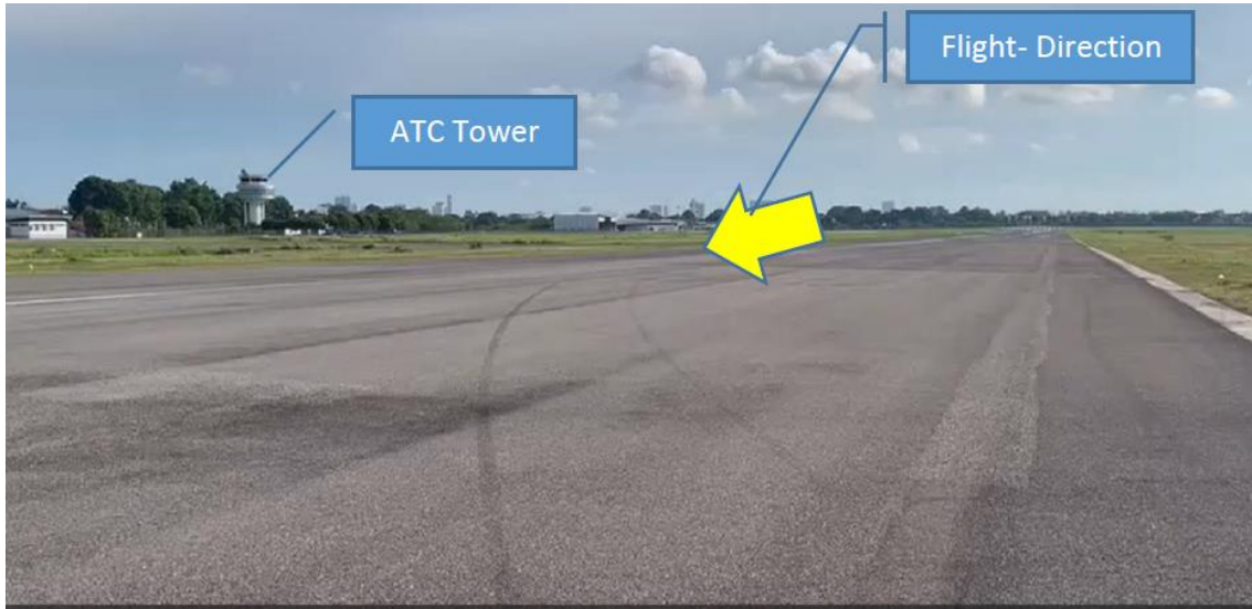
Figure 11: Aircraft tire track marks were observed on the runway at the landing area or exiting the runway towards the crash site.
