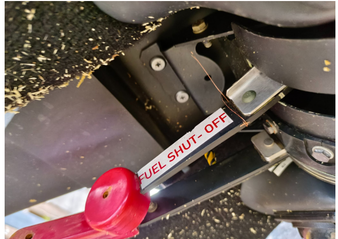
Fuel Shut Off Lever secured with wire and rotor brake off
