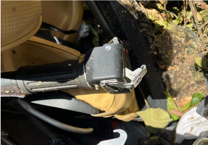
Twist grip at flight position. Collective control unlocked and up midway.
