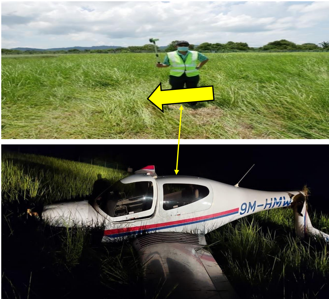
Figure 37: Day & Night - Aircraft final stop position with the broken tail empennage.
