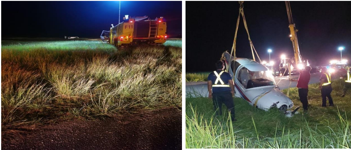
Figure 24: Night – Evidence Limitation: Aircraft skid marks and grass foliage evidence around the first impact point to aircraft final stop position were mostly lost due to rescue work by AFRS vehicle and wreckage salvage work by heavy lift crane and personnel movement. Nevertheless, first impact point and final aircraft rest position can be identified clearly.
