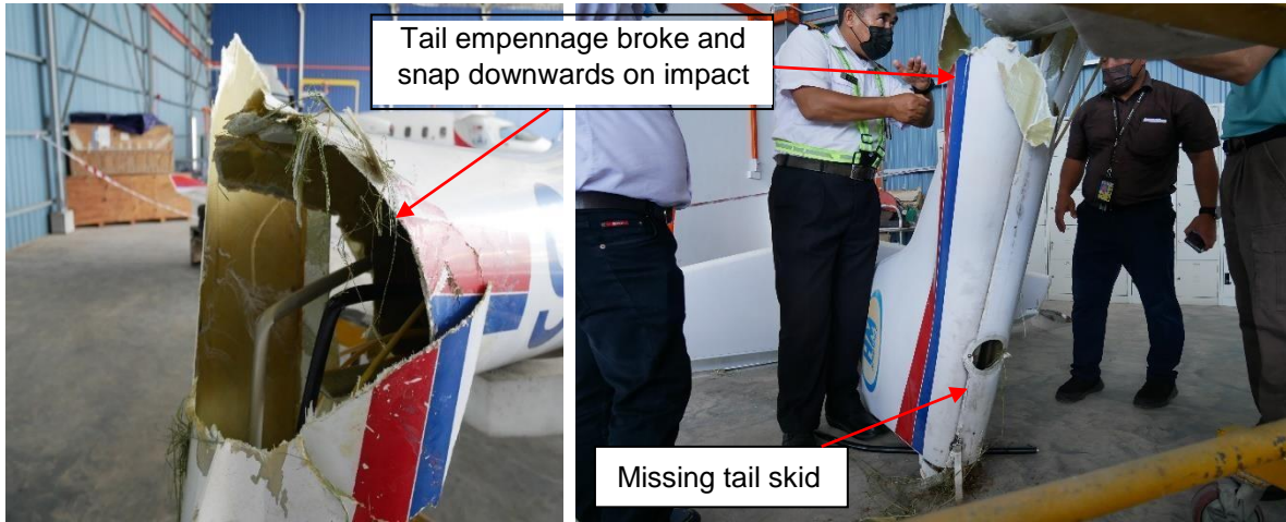
Figure 31: Day - Tail empennage broke and snap downwards on impact. The aircraft tail skid was missing and found near the first impact point area.
