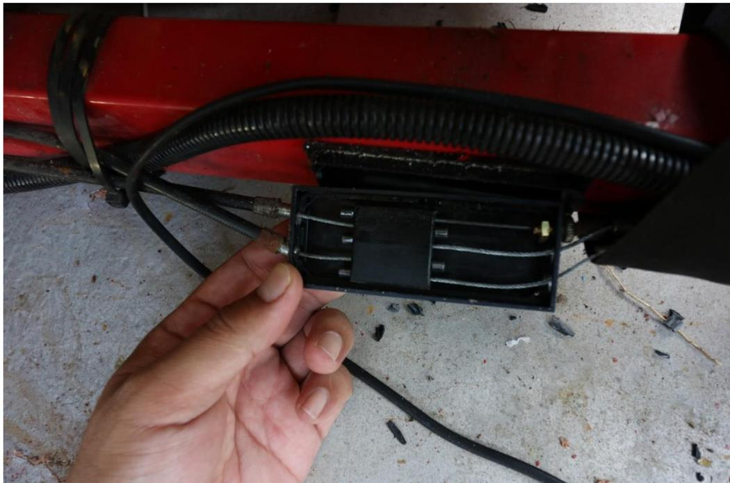
Figure 23: Removing the Throttle Cable
