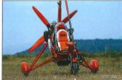
All construction increases greater comfort for our pilots' and passengers' satisfaction. There is an anatomically correct bucket seat which maintains perfect body alignment, a foam headrest and logrest for the rear seat; a new vibration-eliminating motor mount; an ideally placed control bar; adjustable foot rests and pedals and a fork sets on a ball bearing system.
