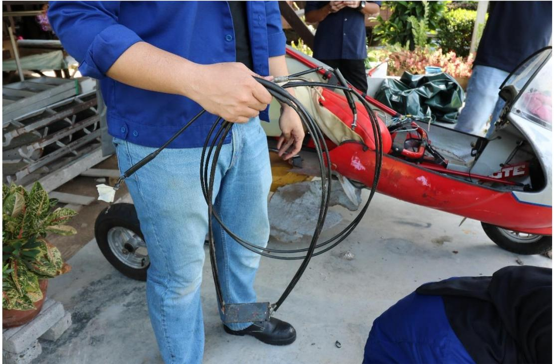
Figure 24: Removing the Throttle Cable
