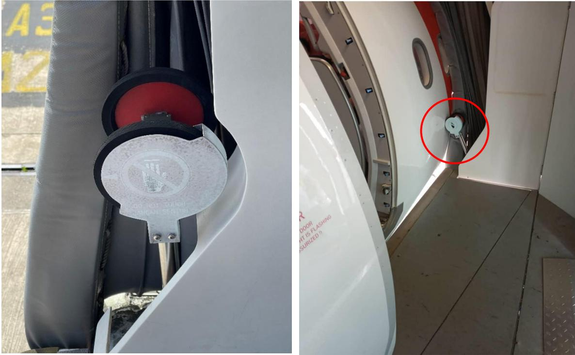
Figure 26: Auto Leveller retracted (Left) and extended to aircraft fuselage (Right) position
