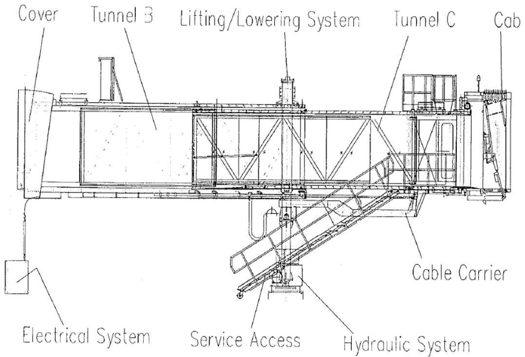
Figure 10: Nosel loader PBB Schematic Diagram
