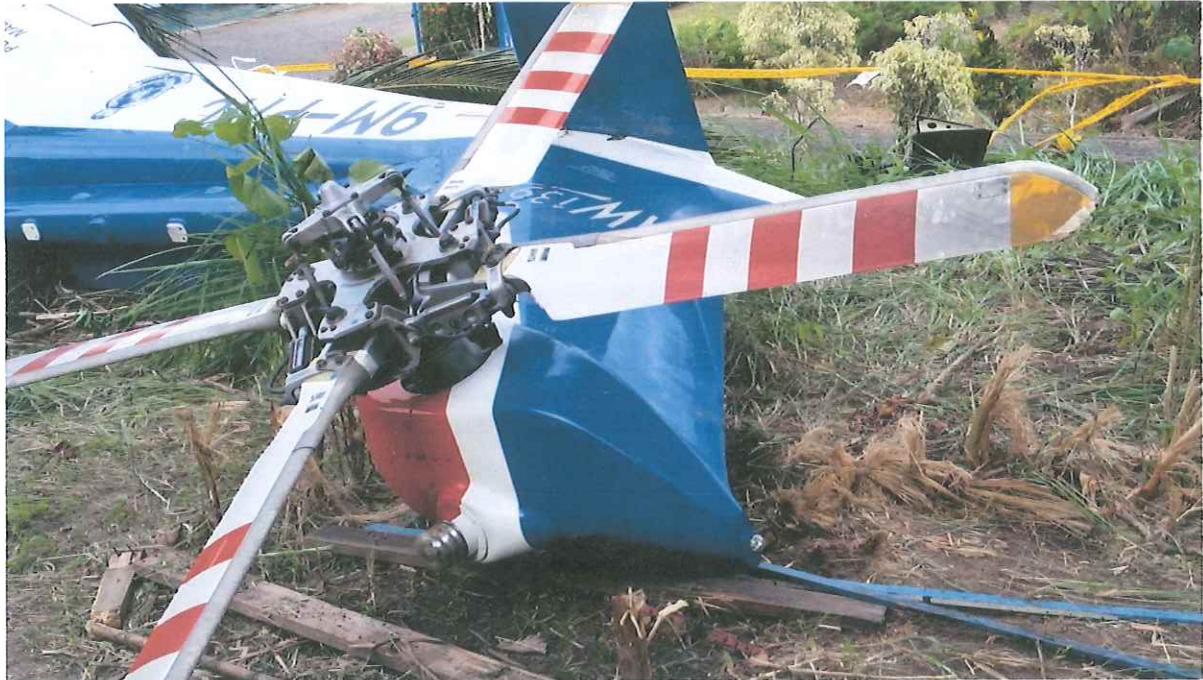
Figure 10: Intact tail rotor system with minor damage at the blade tips
