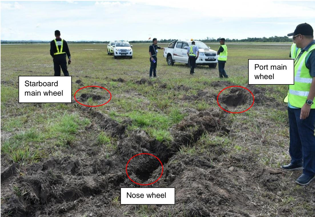
Figure 34: Tyre marks at aircraft final stop position.
