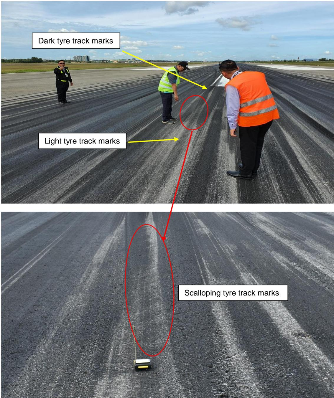
Figure 30: View of the nose wheel tyre track marks near touchdown point. Note how the nose wheel tyre track marks transit from light to dark, increasing in thickness as the veering worsened. The initial scalloping marks indicate possible nose wheel off-set off-centre during landing.
