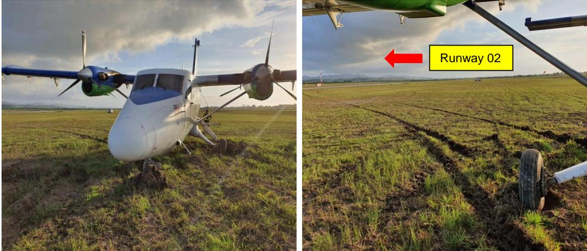
Figure 2: Aircraft final position and skid marks from runway edge
