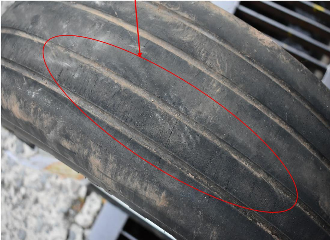
Figure 37: Heavy wear spot mark on the nose wheel tyre consistent with scalloping marks seen on the runway.
