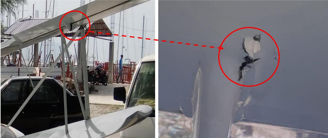
Figure 55: Torn skin underside of the upper right wing aileron fairing most probably caused by an object impact when right wing dropped and impacted the water
