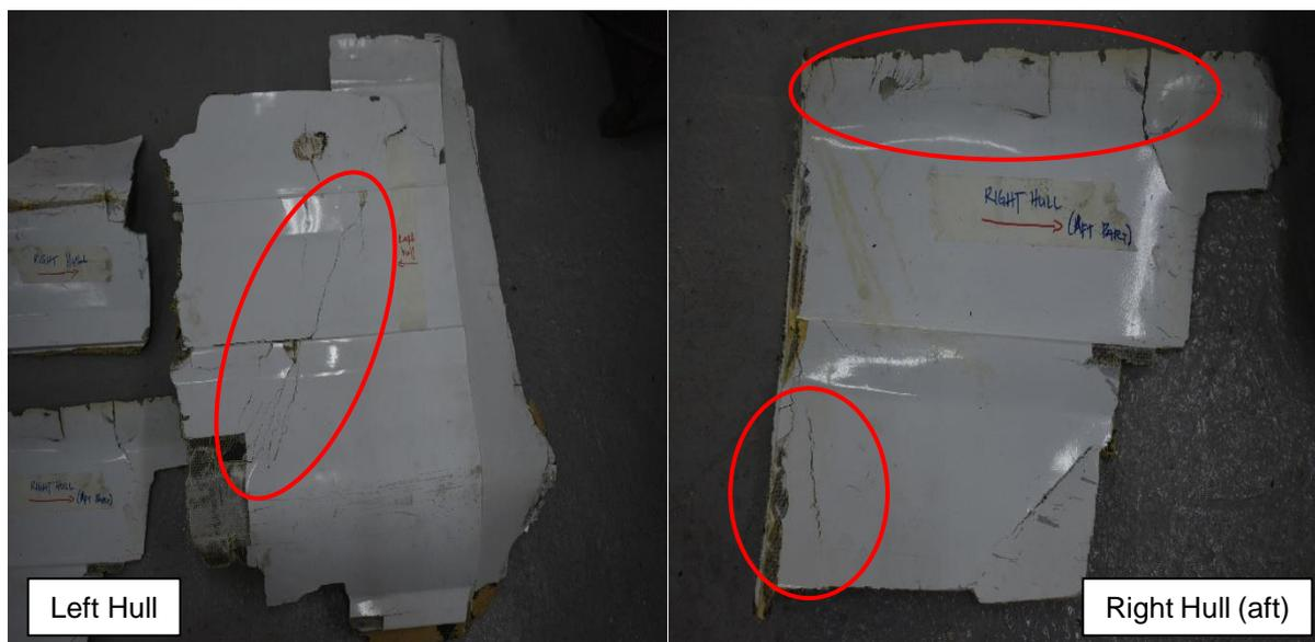
Figure 37: Left Hull and Right Hull (aft) with dented marks and branching cracks
