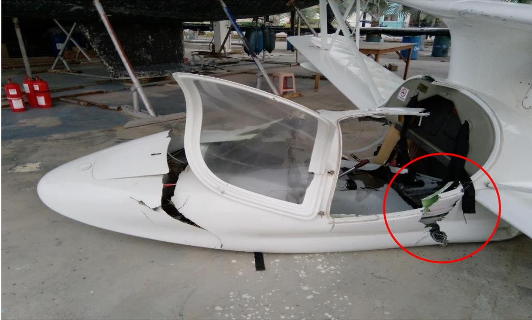
Figure 11: Port Side - Aircraft broke into two through the fuselage and hull just in front of the bulkhead dividing the cockpit and tail section. Window and door are still attached and in relative position. Pilot seat relatively intact.
