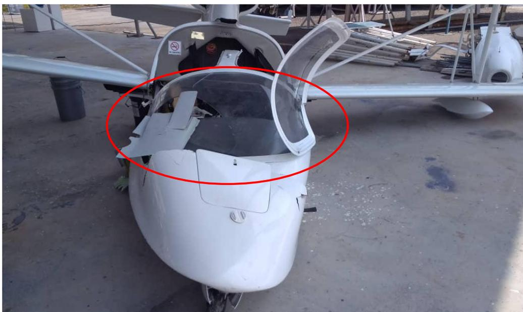
Figure 13: Nose - Damage to the windscreen and nose section during wreckage salvage operations.
