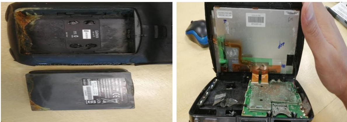
Figure 59: Condition of the GPS after recovery from the wreckage
