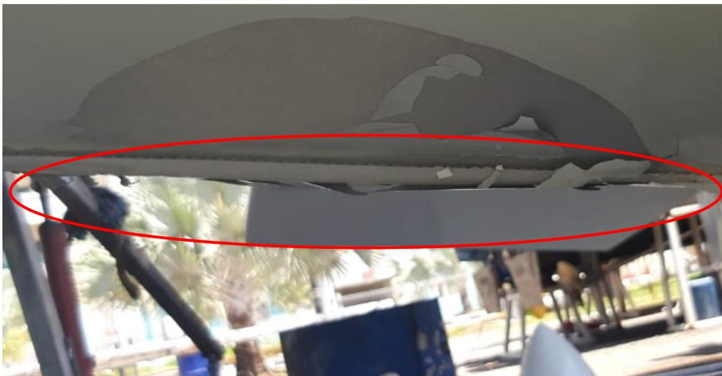
Figure 56: Bulged surface underside of lower right wing most probably caused by water impact at speed when right wing dropped into water creating a dragging force and veering the aircraft to the right
