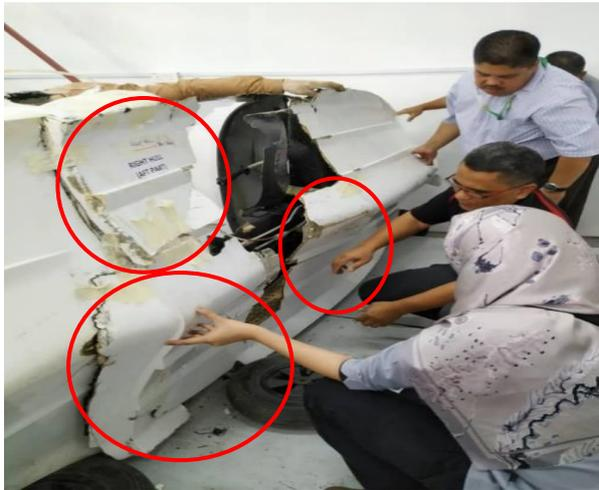
Figure 35: Three main pieces reconstructed to its relative position at the hull section
