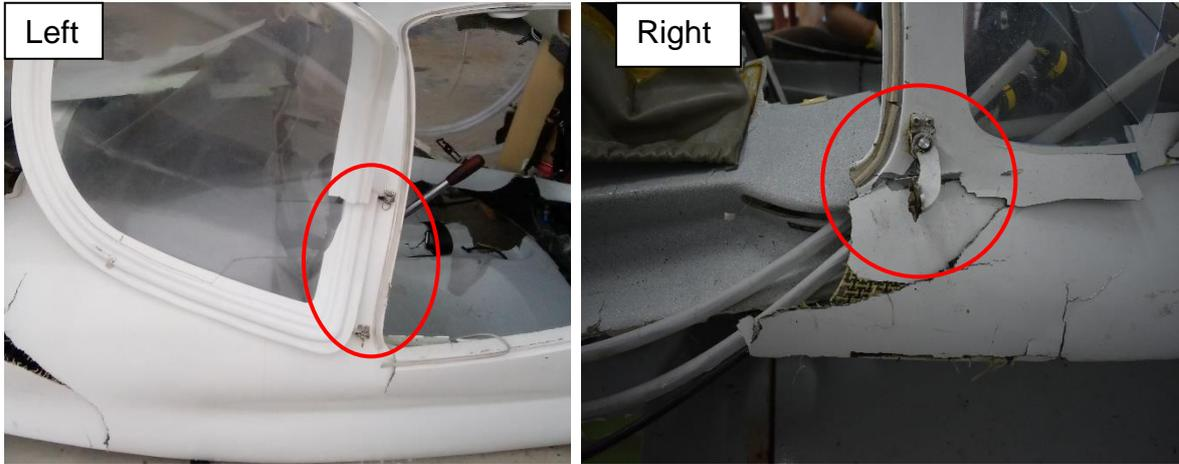
Figure 52: Left window and door hinge still intact
