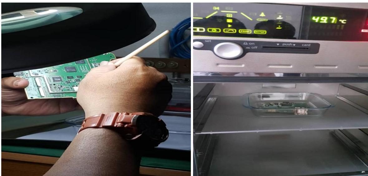
Figure 60: Cleaning and drying process of the GPS PCB at the laboratory
