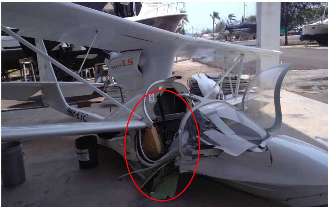
Figure 12: Starboard Side - Fuselage and hull sustained heavy damage with a big tear in front of the bulkhead. Right window and door broke off. Passenger seat broke and collapsed to cockpit floor.
