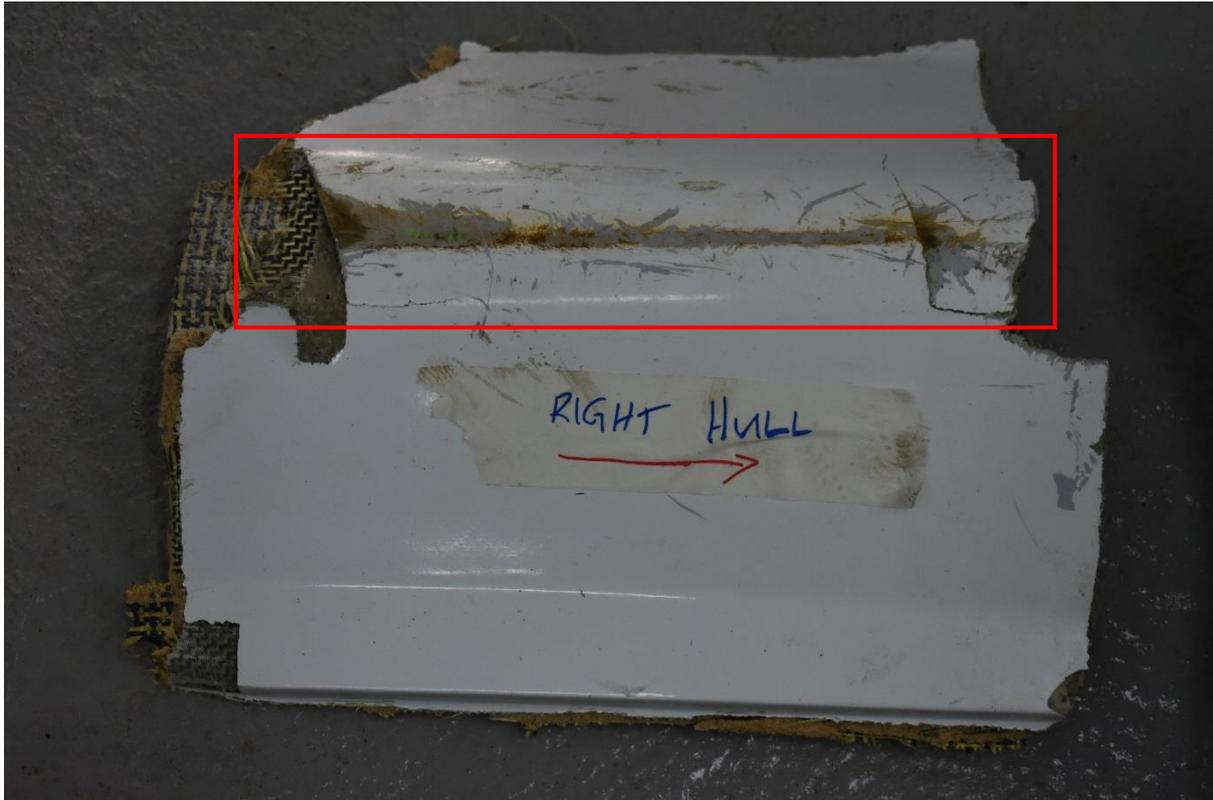
Figure 38: Right Hull with brown trailing impact marks
