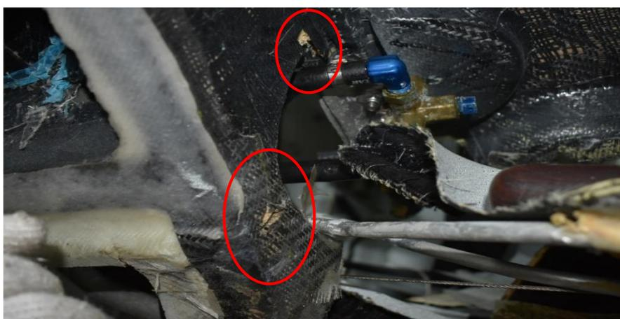
Figure 62: Patched repaired cracks at passenger seat frame still intact after accident (reverse side)
