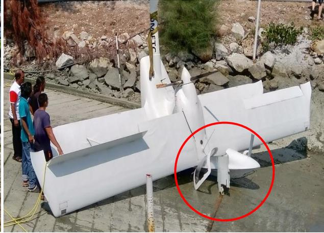
Figure 9: Significant damage to the cockpit and nose section when the aircraft wreckage was lifted and lowered to the upright position by a crane.
