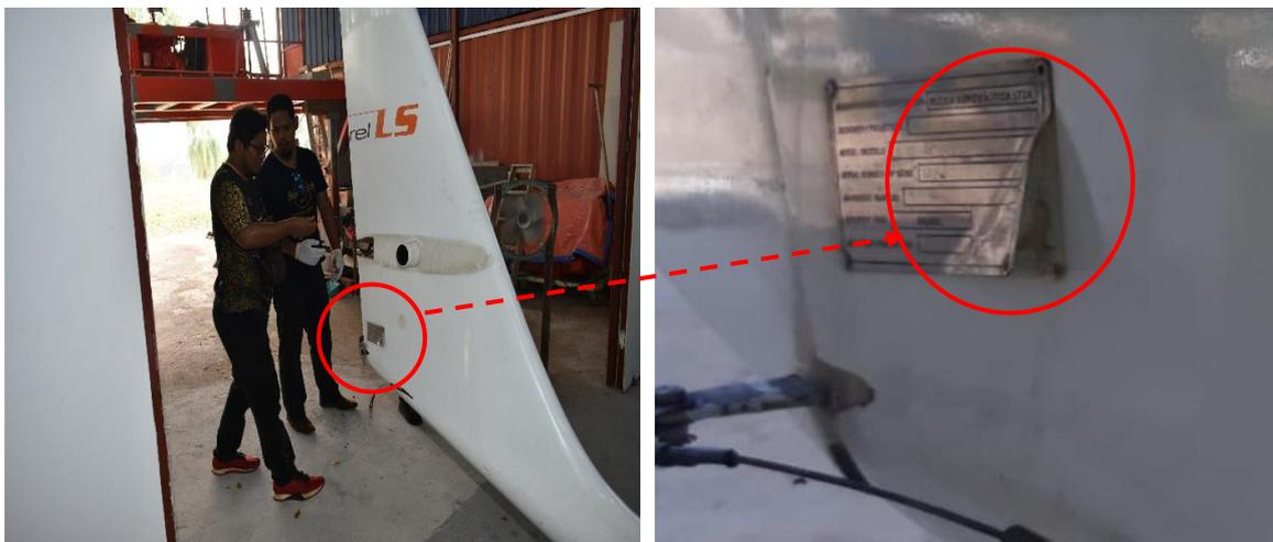
Figure 54: Aircraft registration metal plate on the right tail fuselage section dislodged most probably caused by either boat towing or crank lifting process during salvage operations
