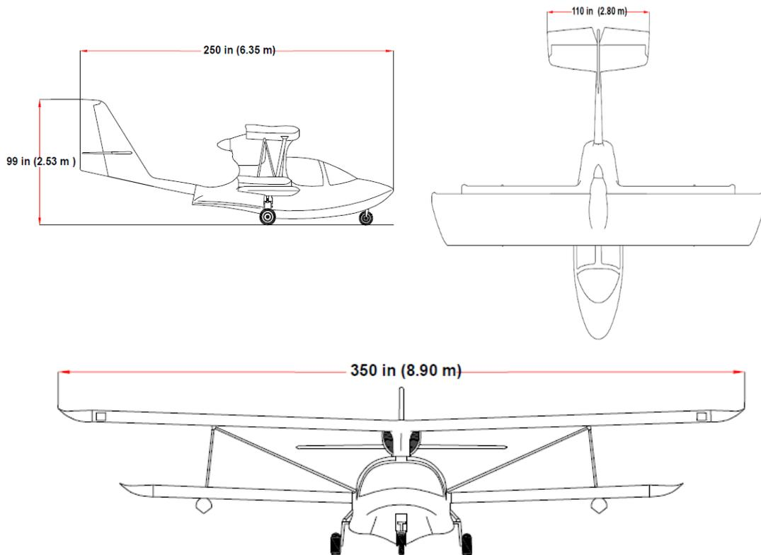
Figure 15: Three View of Aircraft
