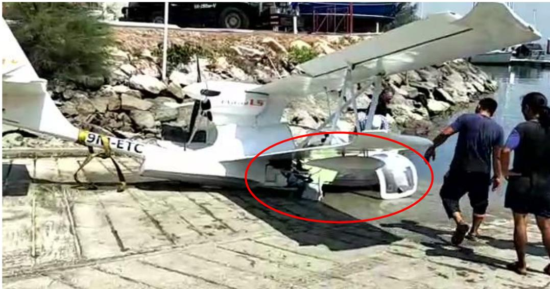
Figure 10: Aircraft wreckage in upright position with fuselage broken into two pieces. Cockpit area and nose section heavily damaged during lowering process by the crane onto the ramp.
