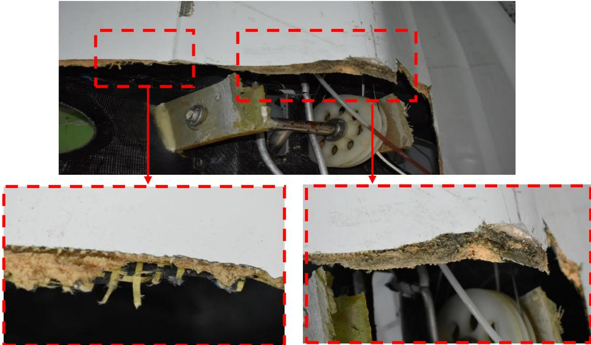
Figure 40: Fractured surface of the hull shows the impact was in the shear and tension mode
