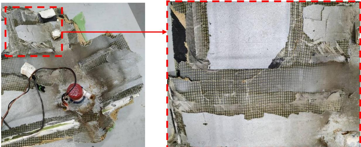
Figure 39: Delaminated & peeled off inner layer of the left hull
