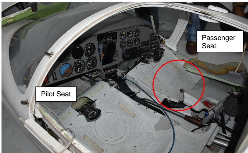
Figure 51: Pilot seat still intact while passenger seat broke and collapsed downward due to broken right hull during impact
