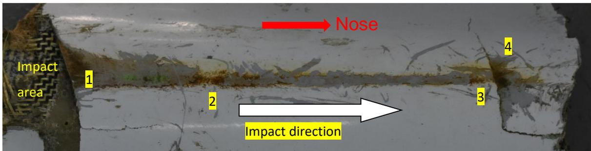
Figure 42: Four (4) selected locations of the impact area (brown trailing mark) marked as number 1 to number 4 for FESEM-EDX mapping analysis
