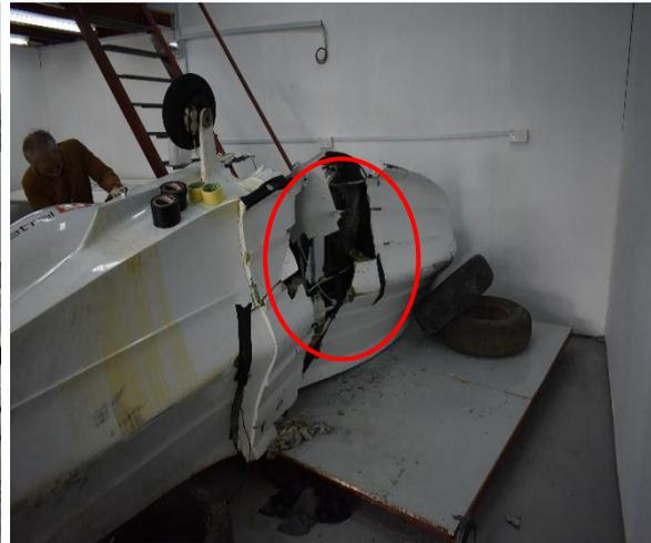
Figure 36: Missing pieces leaving a big gaping hole at the right hull section
