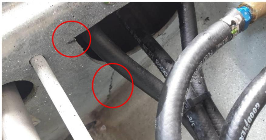
Figure 61: Cracks at passenger seat frame before accident
