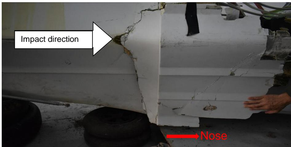
Figure 41: Impact mark on the centre bottom aft hull
