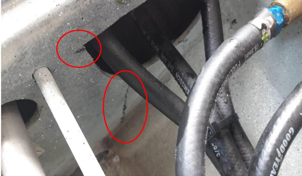
Figure 21: Crack under passenger seat frame.
