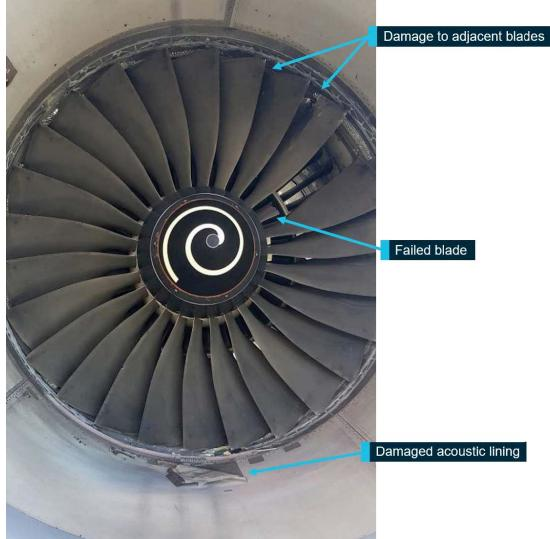
Figure 2: Left engine failed fan blade, with adjacent damaged blades
