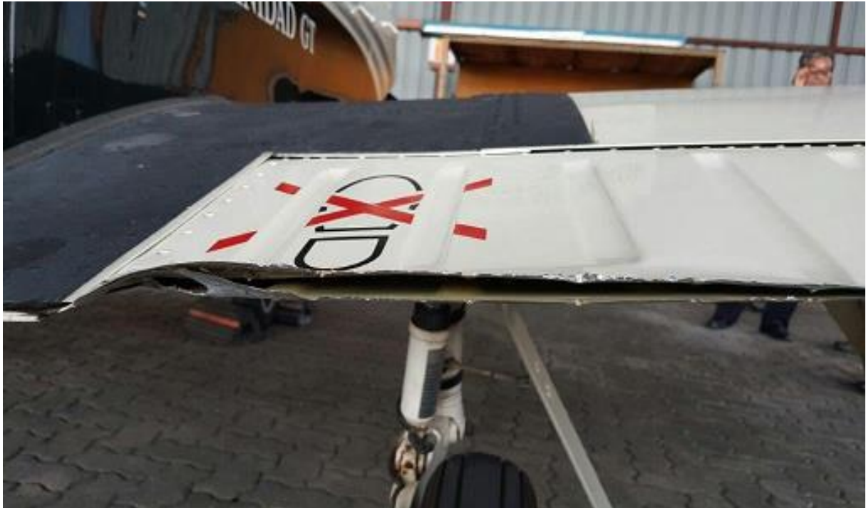
Figure 14 – RH flap damaged
