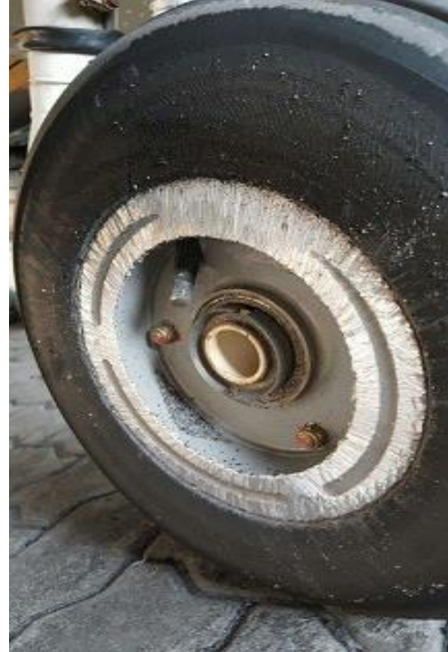
Figure 8 – Wheel hub damaged
