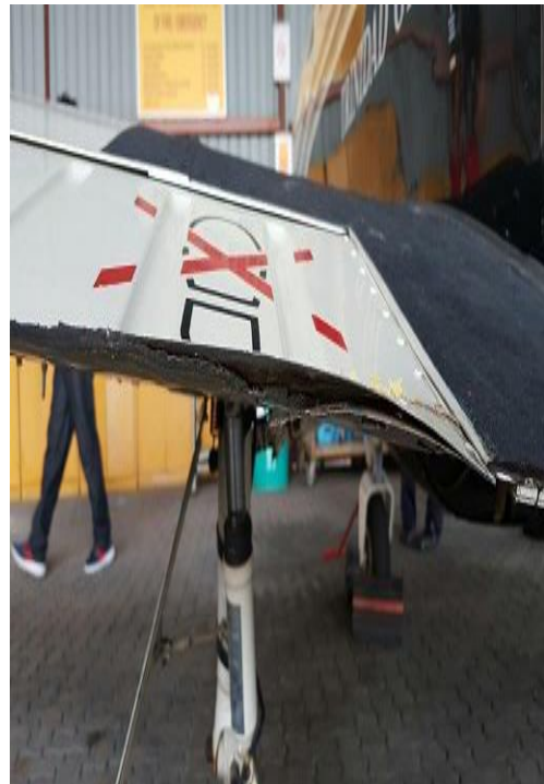
Figure 13 – LH flap damaged
