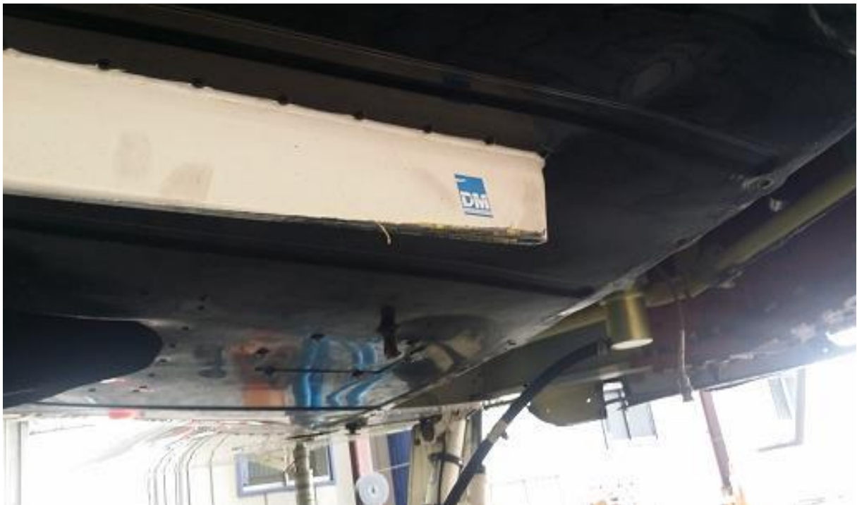
Figure 15 – Bottom antenna scratched
