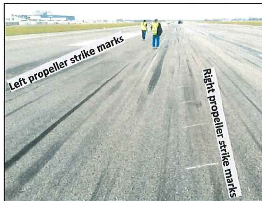
Figure 7. Distance between right and left engines propeller first strike marks (30m)
