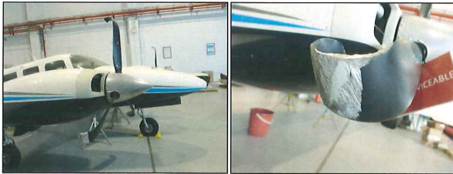
Figure 3. Propeller tip bent forward
