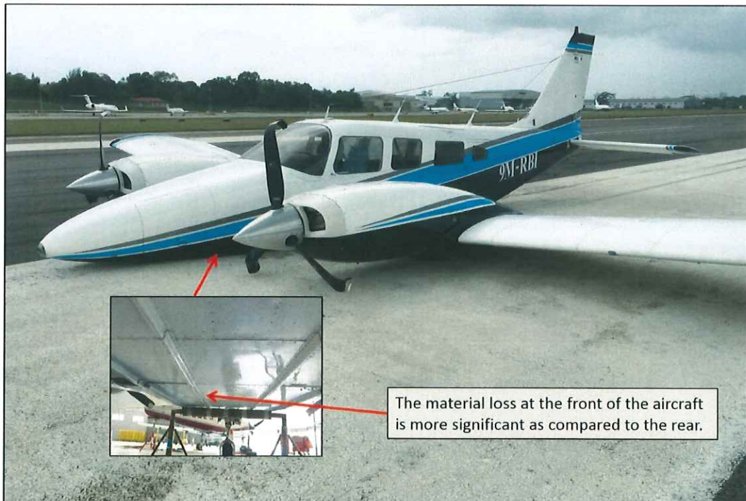
Figure 4. Damage at the belly of the aircraft
