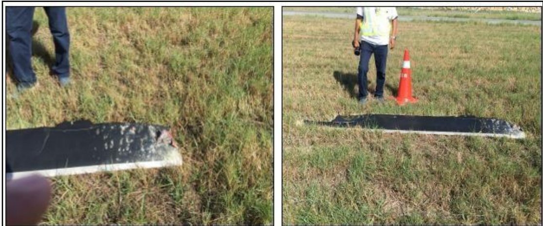
Figure 11: Main rotor blades damage
