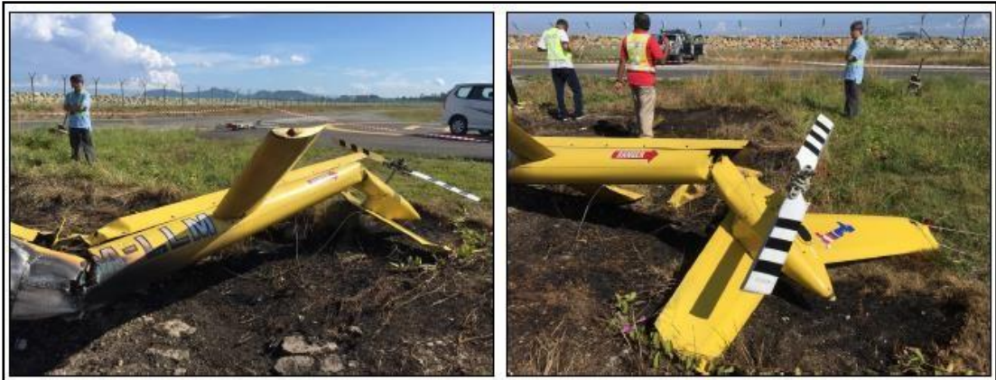
Figure 5: Tail rotor and tail boom condition
