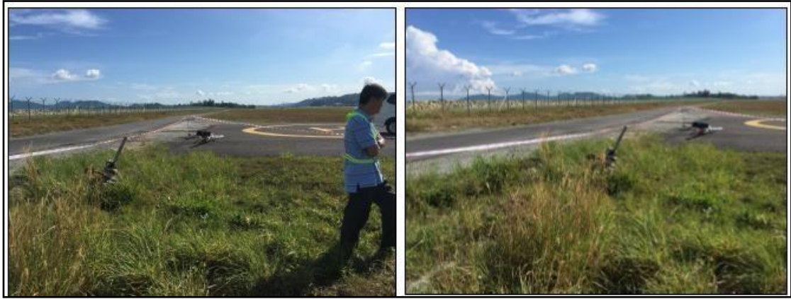
Figure 9: The main gear box detached from the fuselage
