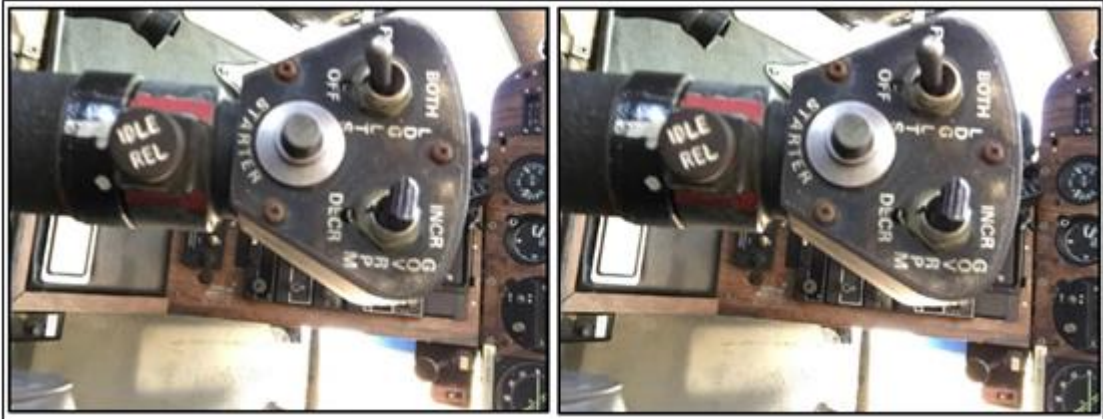
Figure 3: Collective lever and throttle position
