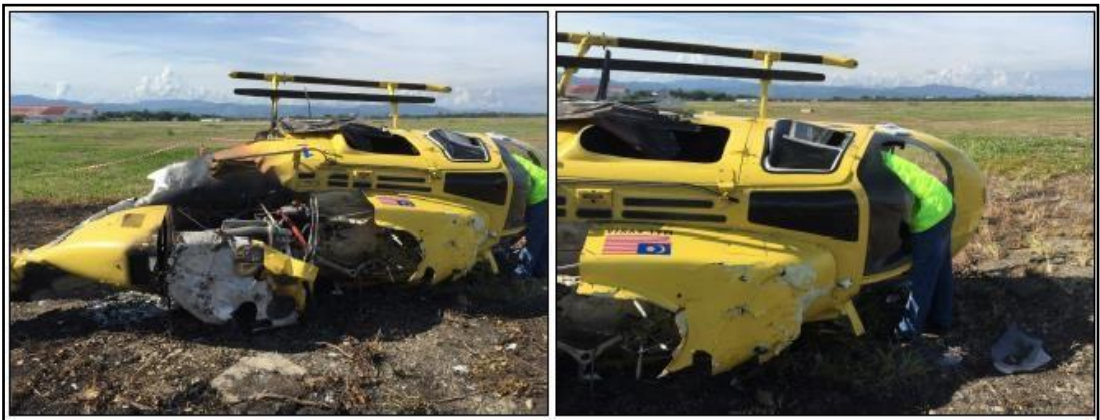
Figure 7: Fire started from the baggage compartment
