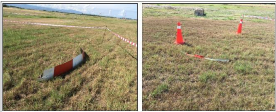
Figure 10: Main rotor broken off due to high rotor energy
