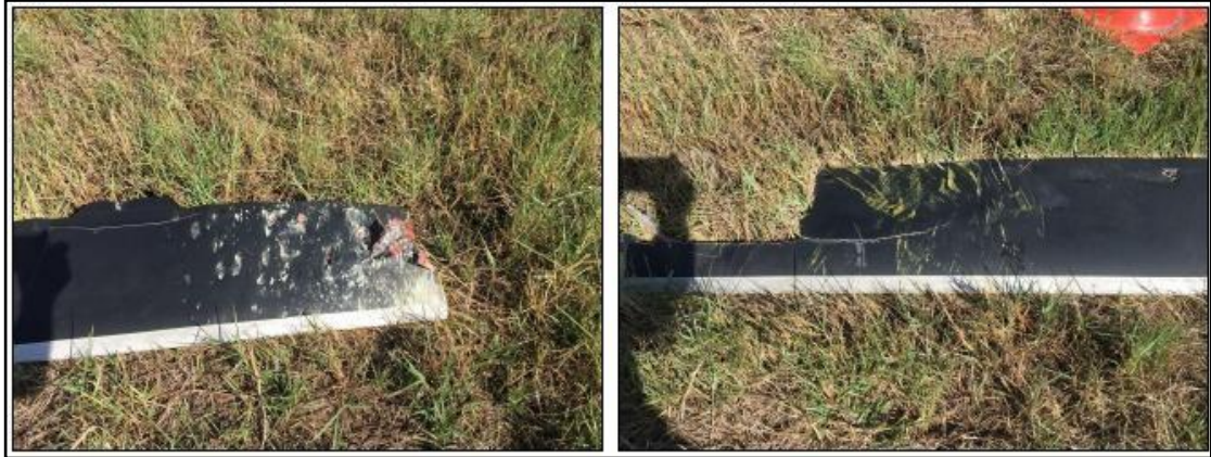
Figure 12: Close look at the main rotor blade tips
