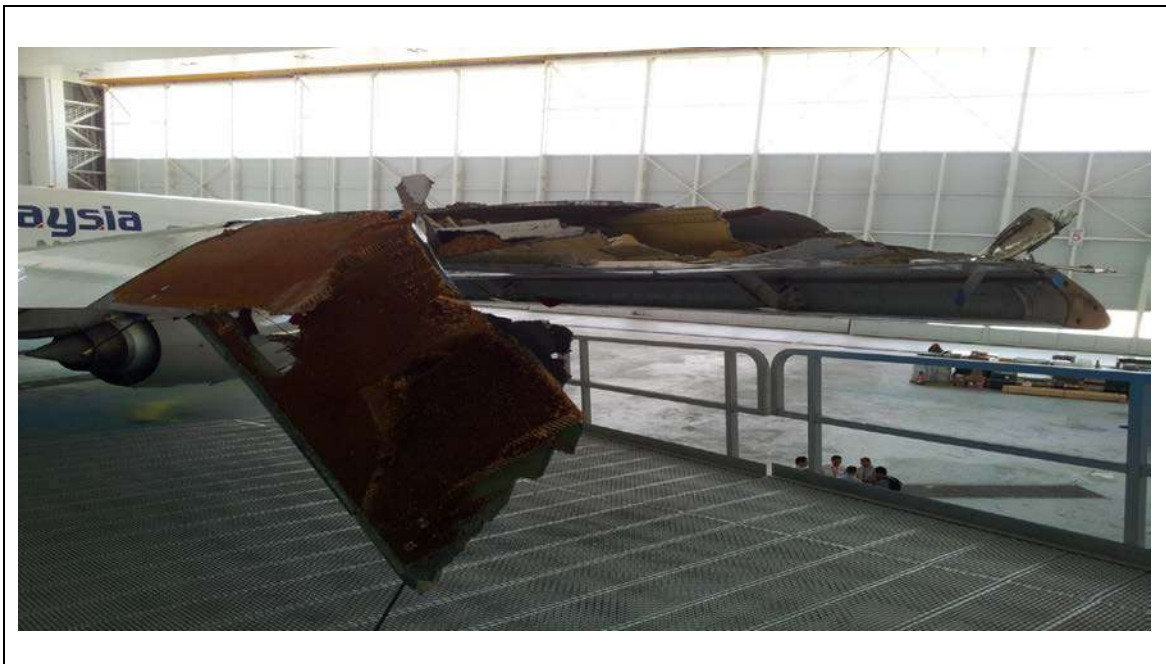
Figure 1.6A - Right Wing Tip Damage
