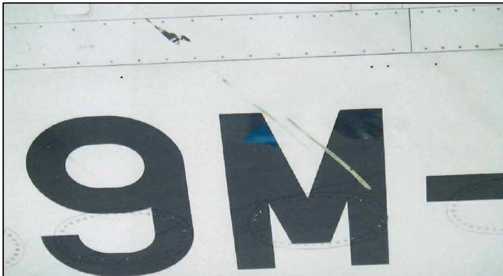
Figure 5: Scratch marks on underside of left wing
