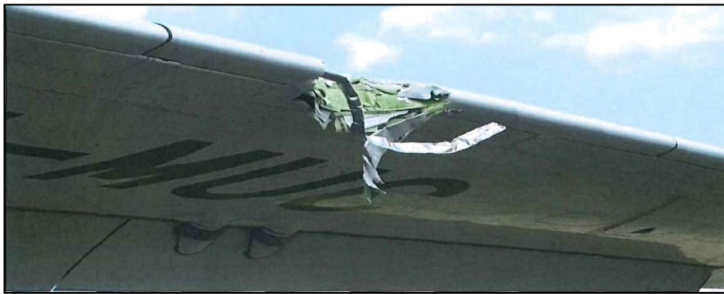
Figure 4: Left Wing No. 6 Stat Damage
