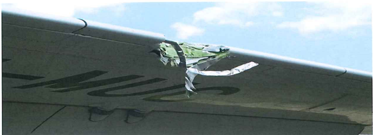
Figure 4: Left Wing No. 6 Slat Damage
