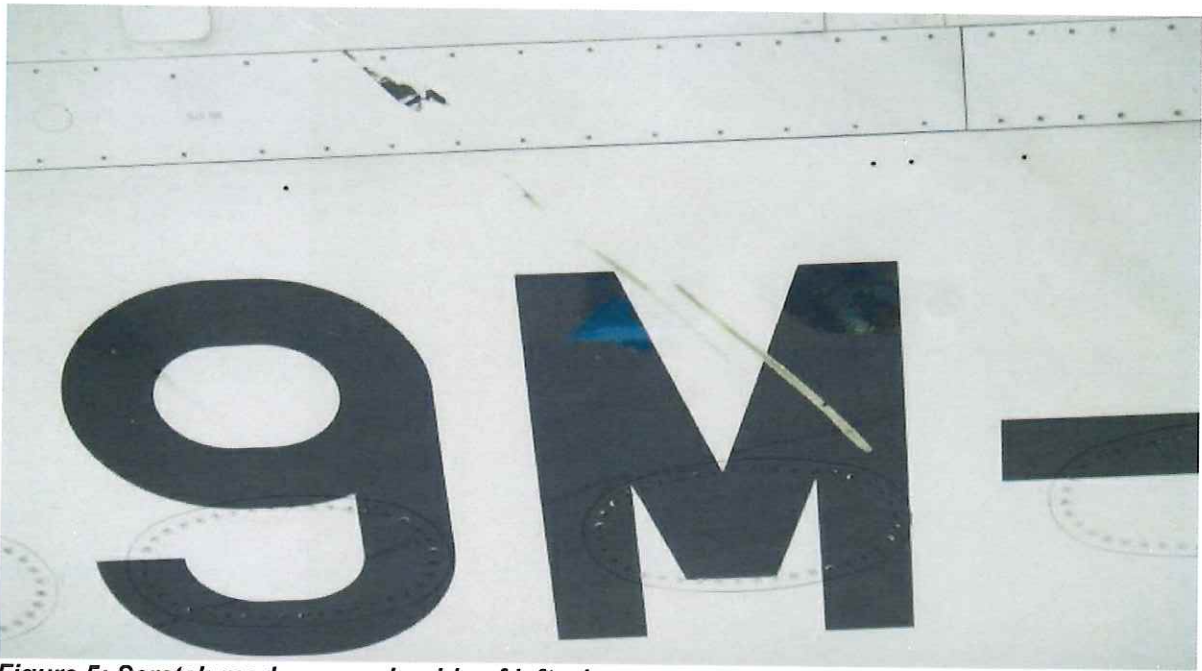
Figure 5: Scratch marks on underside of left wing
