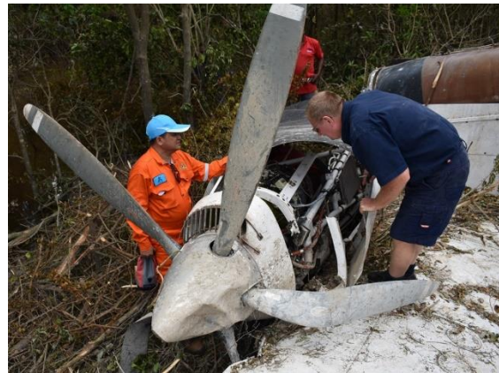
Picture 6 Engine bend to the left
