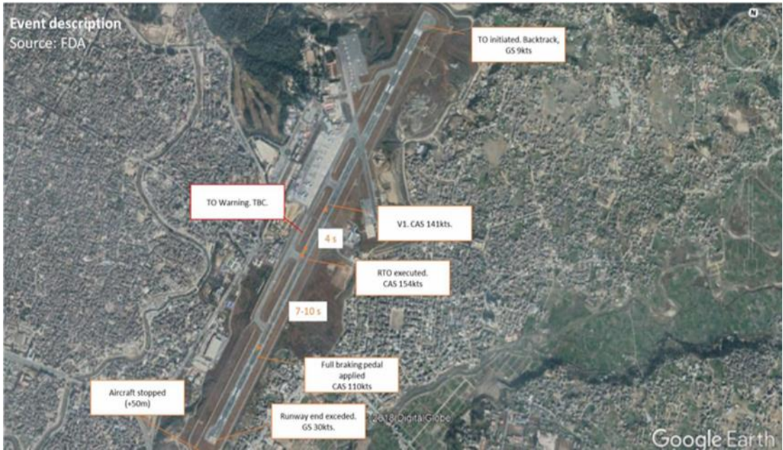
Diagram 2: Sequence of events during take-off roll and RTO (Source FDA/Google Earth)
