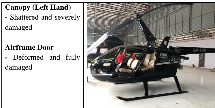
Figure 6: Canopy and airframe door
