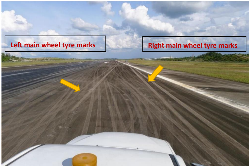
Figure 5: Both main wheel marks show aircraft veering to the right. Left main wheel contacted runway at 620 m from Threshold Runway 13 (shown as “Image 3” in the airport layout in Figure 3)
