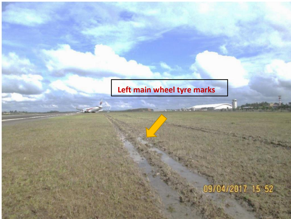
Figure 7: Wheel track on the soft ground approximately 20 m parallel with the runway (Shown as “Image 5” in the airport layout in Figure 3)
