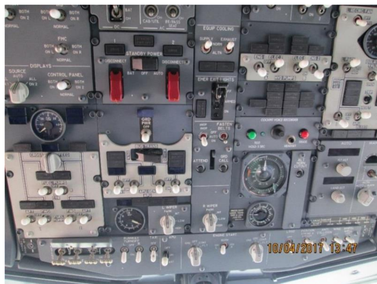
Figure 10: Photograph of Overhead Cockpit P5 Panel
