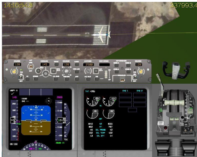
Photograph 1: Aircraft appears to be on the centreline when flying over the Threshold Runway 13 at 42ft RA. No deviation was evident at this juncture.
