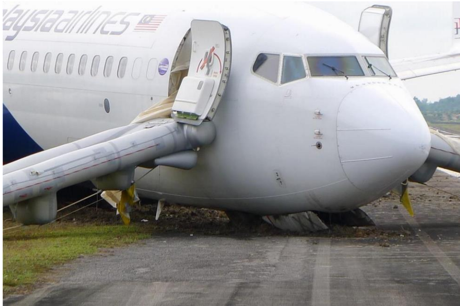
Figure 15: Photograph of Nose Wheel (Collapsed)
