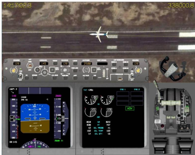
Photograph 7: First point of touchdown (on Right main wheel) at 540 m from Threshold Runway 13. Aircraft heading was 132°. Bank angle was approximately 4° with heading 133°.
