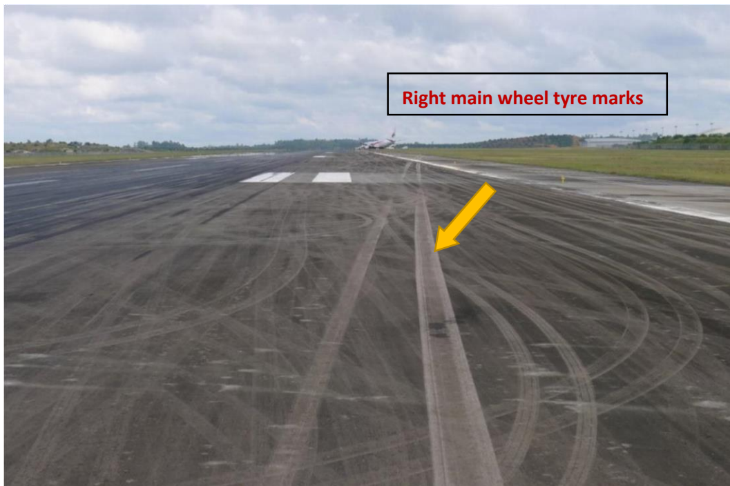
Figure 4: Right Wheel tyre marking on runway (Shown as “Image 2 in the airport layout in Figure 3)
