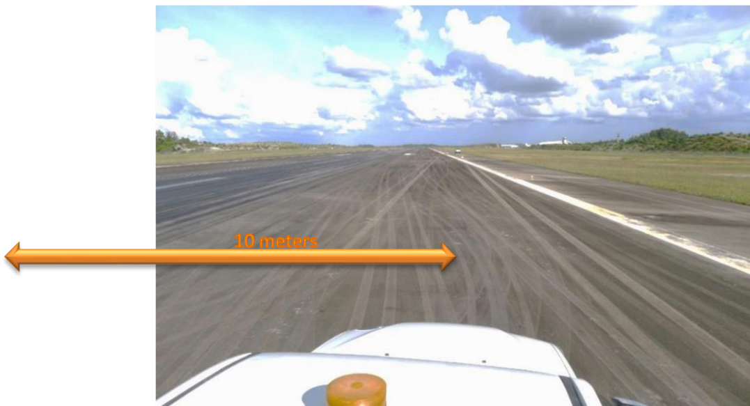
Figure 16: Photograph showing aircraft touchdown position relative to runway centerline.
