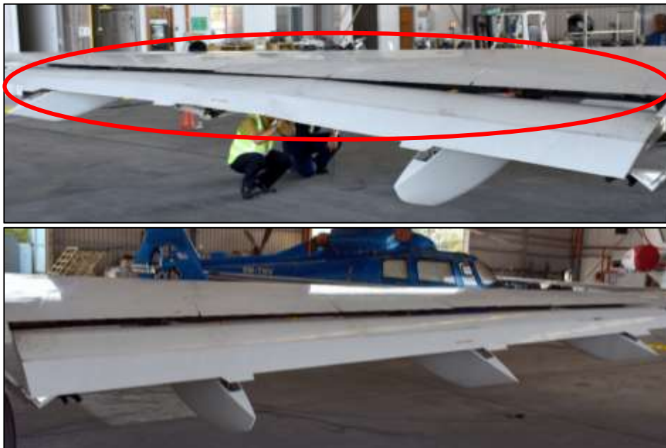
Picture 6 - The flap of the Left Wing was badly damaged as compared to the Right Wing Flap
