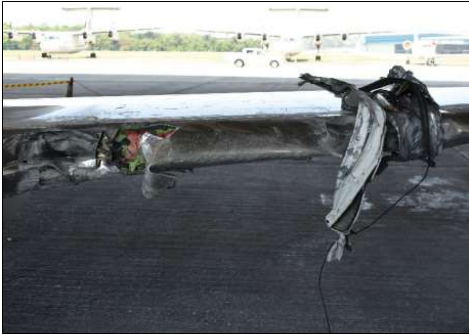
Picture 1 – Mid wing leading edge’s damages with parts of the vehicle Perodua Kembara’s roof stuck to it.
