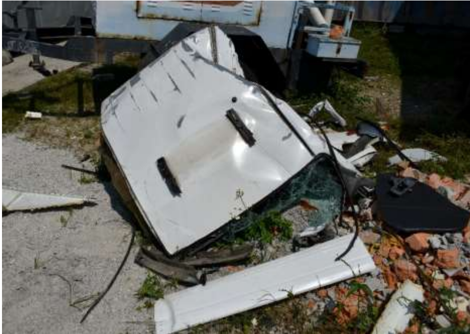
Picture 9 – The roof was totally ripped off from the vehicle
