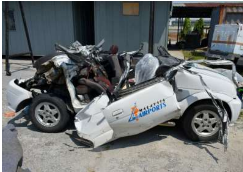
Picture 7 - Perodua Kembara belonged to MAHB AFRS had to cut off and removed the driver's side door in order to remove the victim from the vehicle
